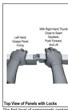
The first level of components contain panel locks that are located at the top of the panel for extra stability and seamless connection. When disassembling panels twist top connection slightly and lift right panel upward.
