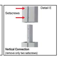
When vertical extrusions are square vertical extrusion using packed in portable cases rather than crates or tubs, they must be broken down into smaller sections which then require assembly.
