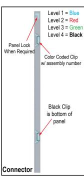
Each component has 2 clips, the lower clip is ALWAYS black. The top clip is color coded to distinguish which level. The color coded clip also contains the numbered label.
