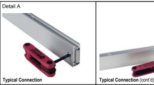
Most horizontal extrusion connections have a patented expandable lock. This lock inserts into the groove of an opposing extrusion. Tightening the lock with the Hex Key Tool expands the lock and creates a strong positive connection.
